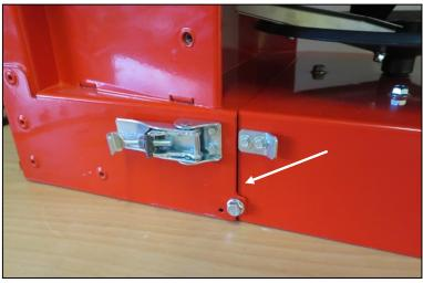
• Now you can still adjust the tension of the two quick-release fasteners (Fig.: 51). To do this, turn the hooks with the thread. To fasten the plate frame, hang the hooks of the quick-release fastener in the hooks of the plate frame on both sides. Then fix the adjustment by tightening the nut on the quick-release fastener.
