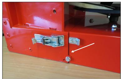
Now you can still adjust the tension of the two quick-release fasteners (Fig.: 135). To do this, turn the hooks with the thread. To fasten the plate frame, hang the hooks of the quick-release fastener in the hooks of the plate frame on both sides. Then fix the adjustment by tightening the nut on the quick-release fastener.
