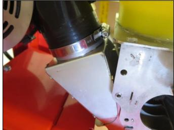
Now install the air channel from the bottom through the large opening and fasten it on each side with one hexagon bolt (marked in Fig.: 81).
