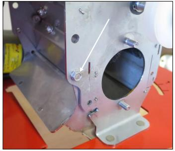
• To install the seeding shaft motor cover, position it from top to bottom **1** over the seeding shaft motor and fasten it with the existing bolts 2 (Fig.: 101).
