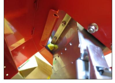
• Install the transition pieces from the bottom in the direction shown by the arrow 1 onto the air channel and fasten them on both sides with one quick-release fastener 2 each (Fig.: 84).
