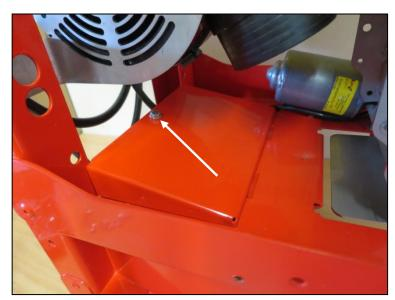
• Now disconnect the cable for the blower fan from the terminal strip. It is connected on the left side of the terminal strip in Fig.: 45 (see also the connection diagram, page 23, Fig.: 46).
