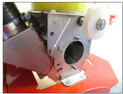
• Loosen the hose clamp marked in Fig.: 17 to remove the transition piece from the metering unit to the blower fan (Fig.: 18). Then remove the hose clamp from the blower fan.
