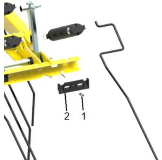
Figure 18: 1 = nut, 2 = plastic piece
